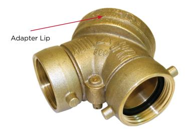
This procedure involves installing one or more 5/16-18 Allen set screws as well as a special permanent adhesive in order to secure FDC Brass to the pipe thread on the building. This will minimize the chance of theft.
